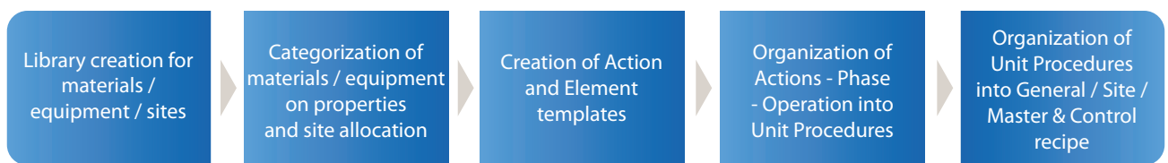
Figure 4a: Recipe Re-Structuring Using PLM Platform Aligned to ISA-S88 Standard
