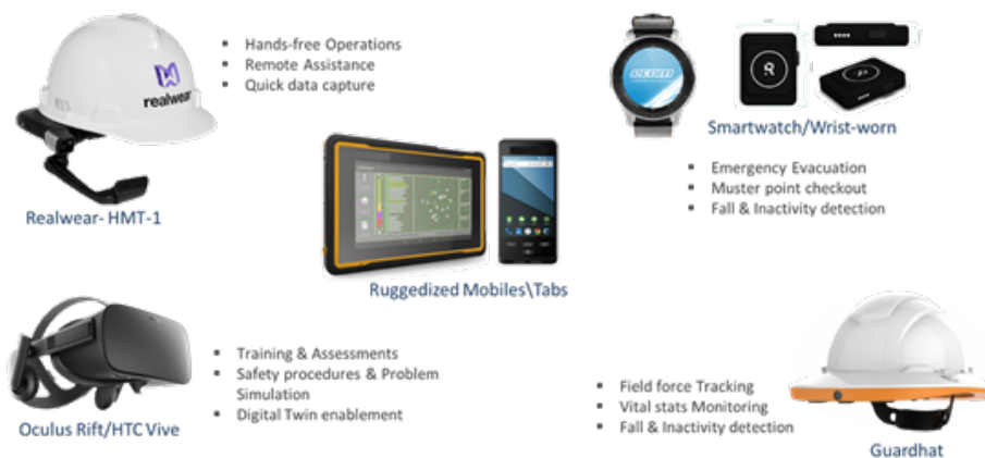
Examples of Wearables and Handheld Devices That Enable the Connected Worker in Industry (Source: TCS)
