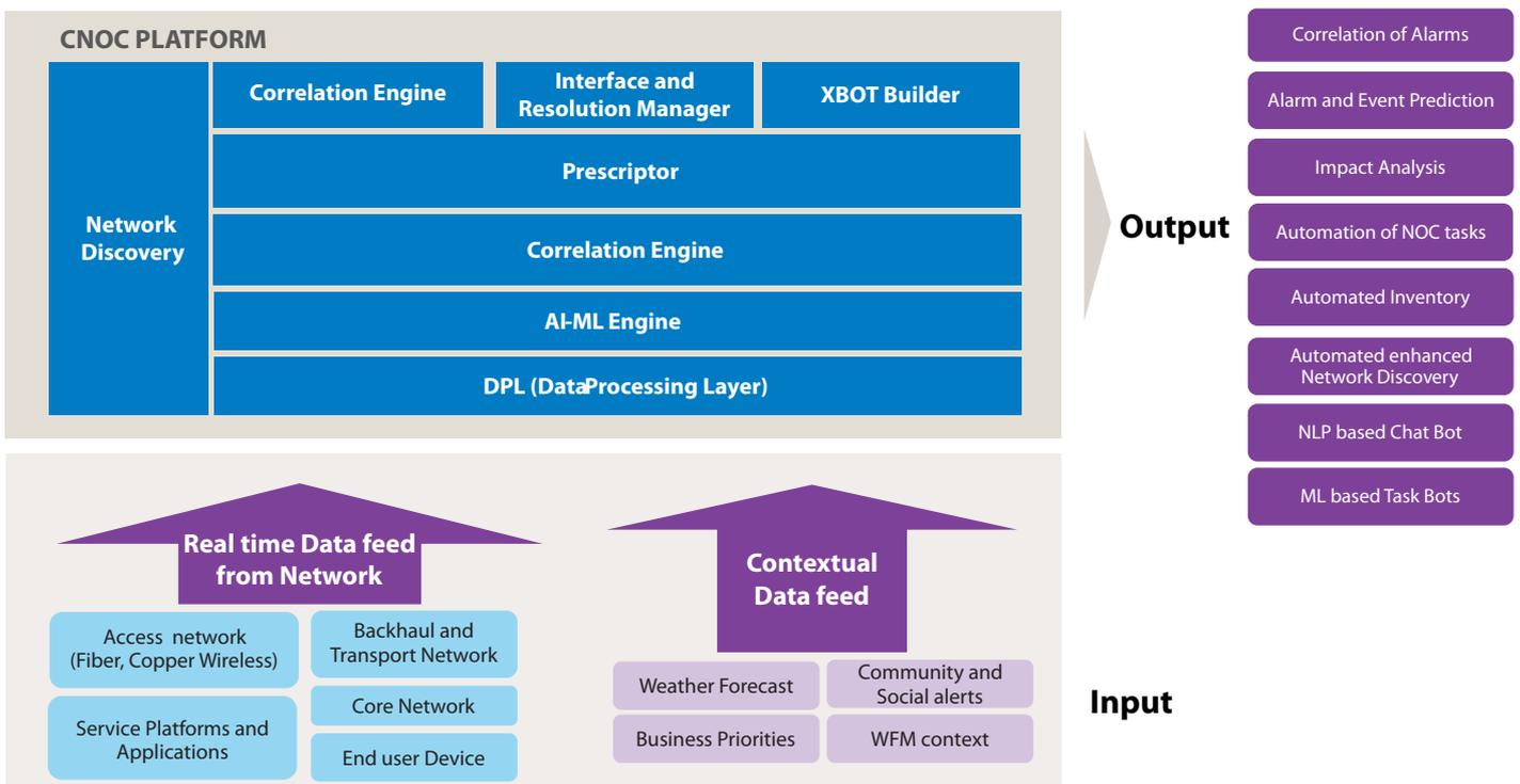
**Figure 1: Three-layered framework of a cognitive NOC**
