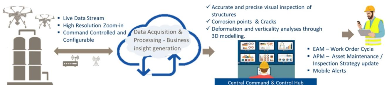
Figure 3: HSSE risk reduction in storage tank inspection
