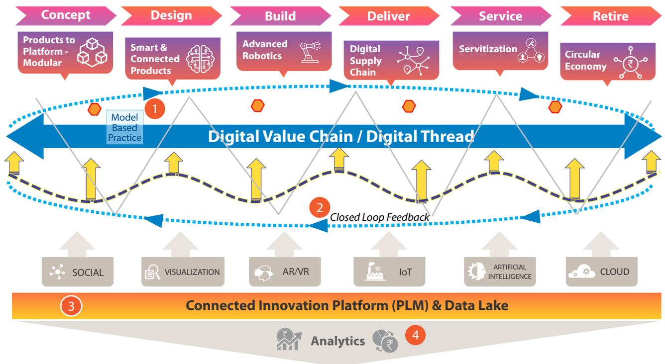
Figure 1: The key constituents of digital thread
