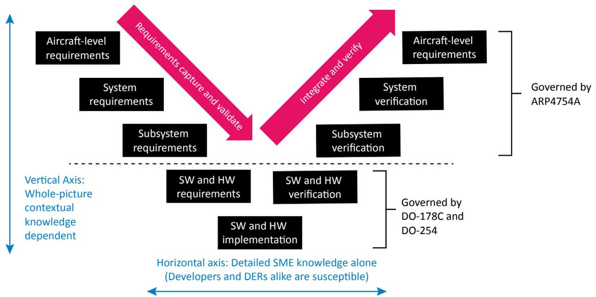
Figure 1: FAA-accepted model for development and certification of complex systems
