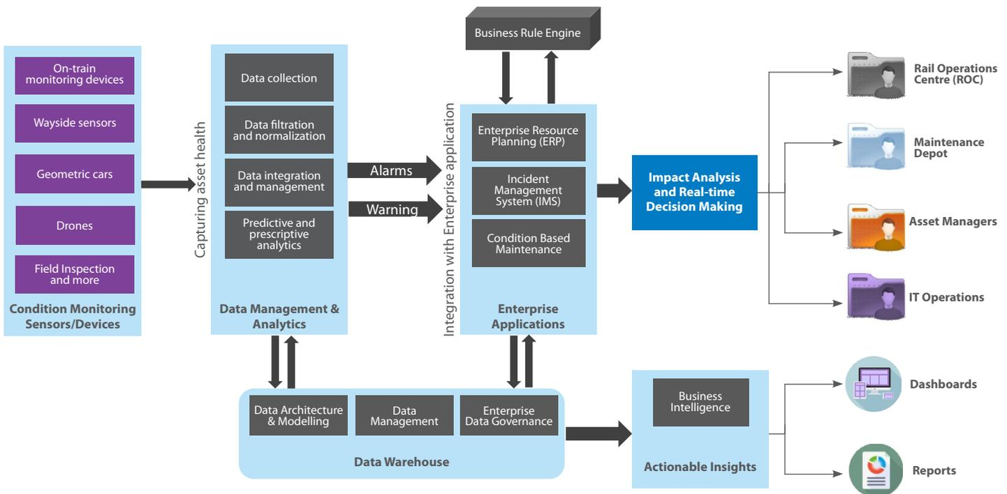
Figure 1: High-level View of IoT-based Predictive Maintenance Solution
