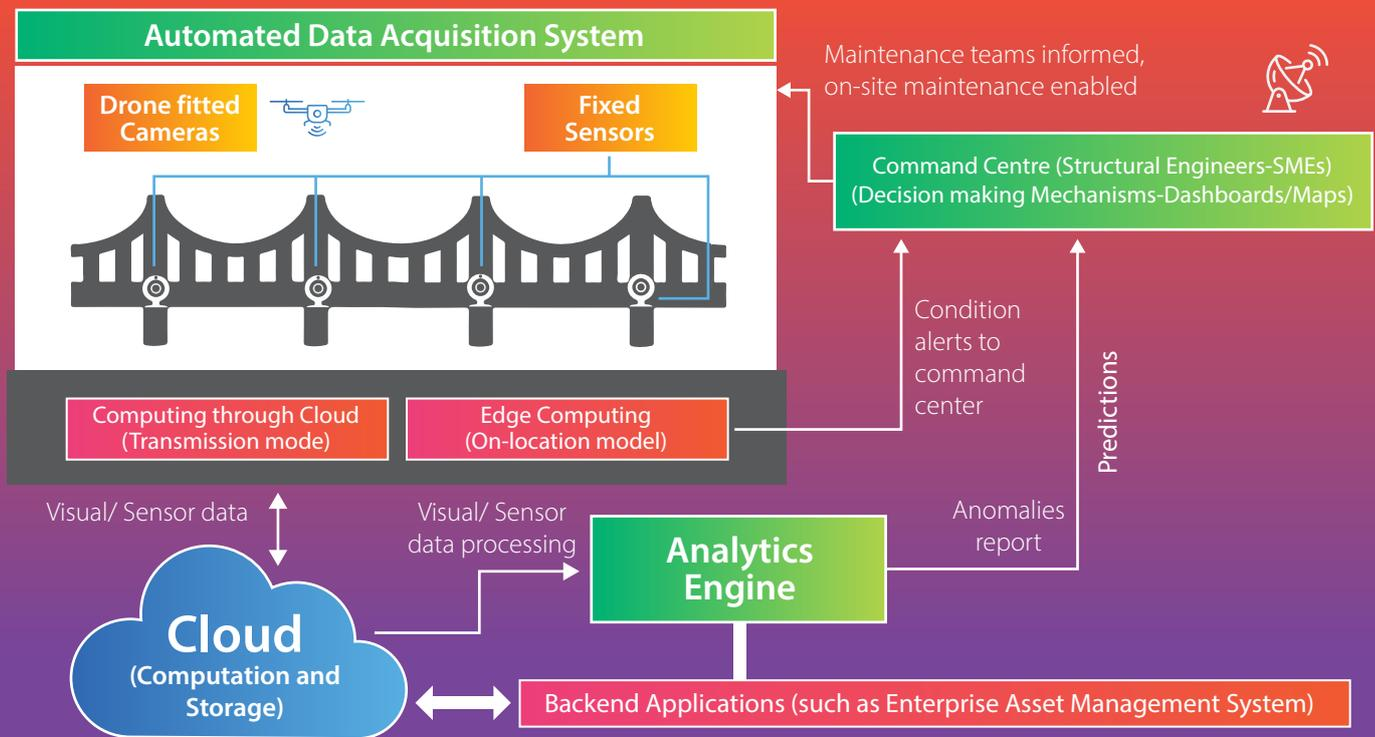
Figure 1: Rail Bridge Inspection Automation
