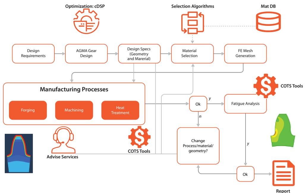
**Figure 3:** Process for gear design and manufacture
