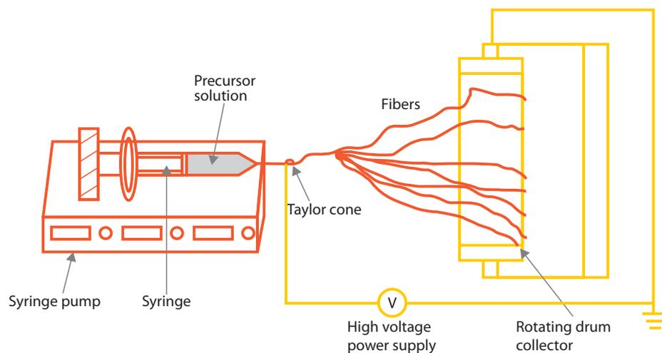
**Figure 2:** Schematic of synthesis of nanofibers by electrospinning
